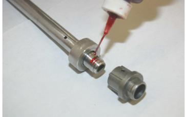
Loctite & reinstall damping rod head, re-install cut down roll pin portions to secure.
