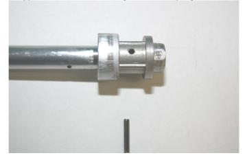
Remove roll pin & cut down so as not to block oil flow thru center of damping rod
